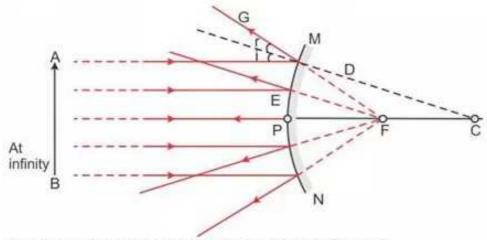
(ii) Concave mirror converges a beam of light falling on it.
