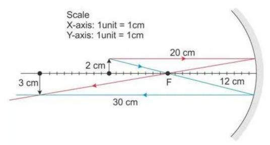
The image is 30 cm in front of the mirror, 3 cm high, real, inverted and magnified.
