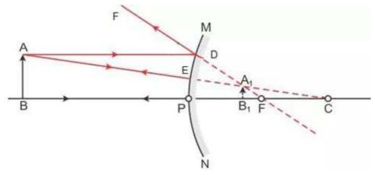
The image formed is virtual, erect and diminished.
