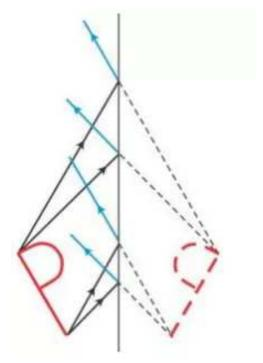
Figure above shows the image formation of a letter P in a plane mirror.
