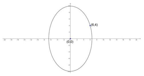
Let us assume the equation of the ellipse is  $\frac{x^2}{a^2} + \frac{y^2}{b^2} = 1 - - - (1)$  (a<sup>2</sup><b<sup>2</sup>), since centre is at origin and foci on y - axis.
