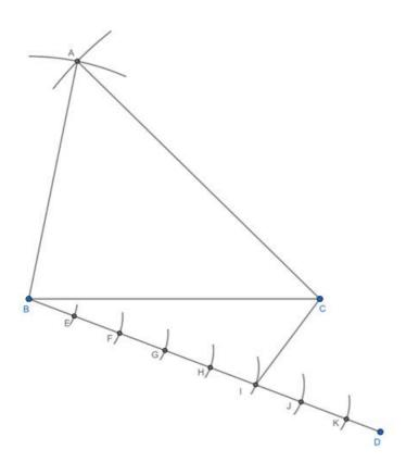
4) Taking I as the center and any radius, draw an arc., intersecting BD and Cl at L and M respectively. Taking K as the center and radius IL, draw an arc., intersecting BD at N. Taking N as the center and radius LM, draw an arc, intersecting previous arc at O. Join and extend KO, intersecting extended BC at P.
