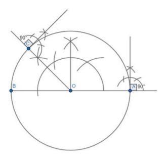
Step 3: We construct perpendiculars to OC and OA at points C and A respectively.
