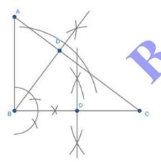
Step 3: Construct perpendicular bisector of line segment BC, which intersects it at pt. O.
