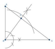
Step 2: Construct a perpendicular from point B onto AC. Point D is where this perpendicular meets AC.
