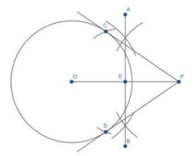
Step 5: We join points P and C, and P and D to get tangents PC and PD to the circle.
