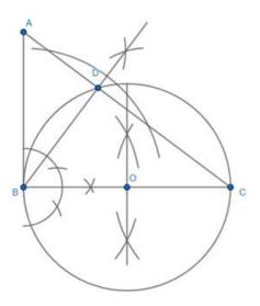
Step 4: Taking centre at O and radius as OB, we construct a circle. It passes through points C and D too.
