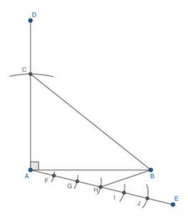
4) Taking H as the center and any radius, draw an arc., intersecting AE and BH at K and L respectively. Taking J as the center and radius HK, draw an arc, intersecting AE at M. Taking M as the center and radius KL, draw an arc, intersecting previous arc at N. Join and extend JN, intersecting extended AB at O.
