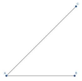
Step 1: Draw a line segment AC of arbitrary length and at an any angle to AB such that ∠CAB is acute.
