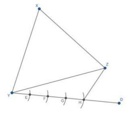
3) Taking H as the center and any radius, draw an arc., intersecting YD and ZH at I and J respectively. Taking G as the center and radius HI, draw an arc., intersecting YD at K. Taking K as the center and radius IJ, draw an arc, intersecting previous arc at L. Join and extend HL, intersecting YZ at M.
