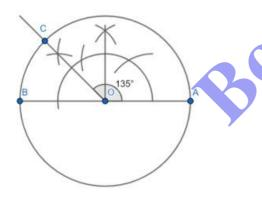
Step 2: We construct an angle of 135° at centre O, such that  $\angle AOC = 135^{\circ}$ , where C is another point on the circle.
