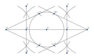
Step 5: We join points P and K, P and L, Q and M, and Q and N to get the tangents PK, PL, QM, QN from points
