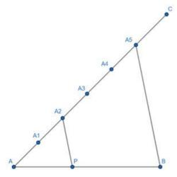
Step 4: We draw line segment  $A_2P$  such that  $A_2P \parallel A_5B$  and P is the point of intersection of this line segment with AB.
