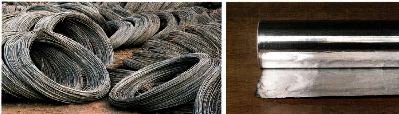
Fig. 6.2 Metals are ductile and malleable—they can be drawn into wires or pressed to form sheets or foils.
