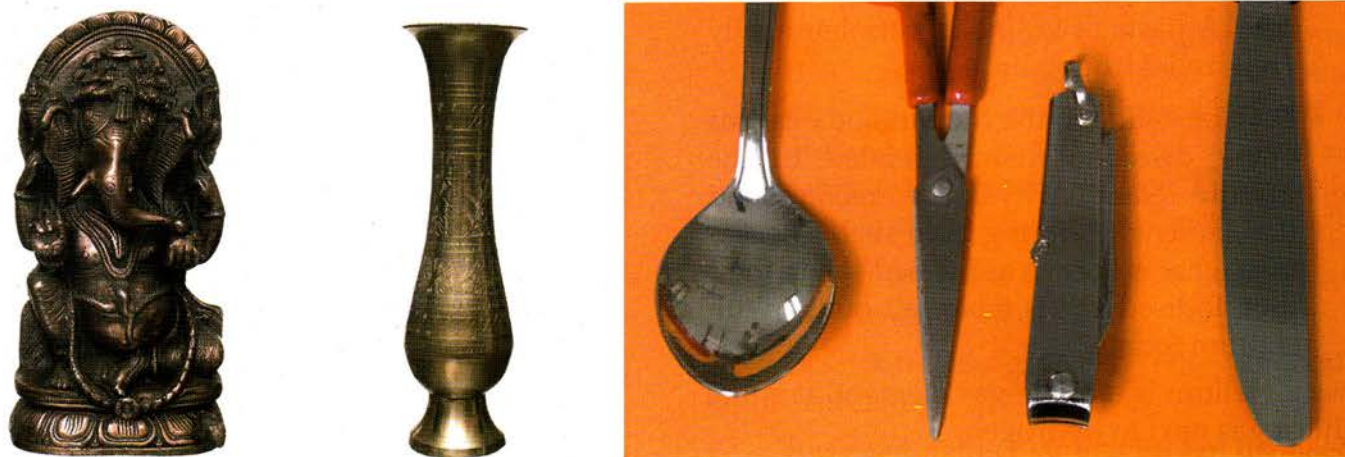
Fig. 6.7 A bronze statue, a brass vase, and things made of stainless steel
